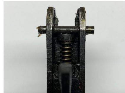
Figure 2 - Spring where MagLatch is to be installed.
